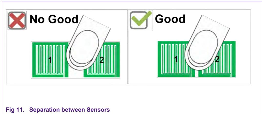
Fig 11. Separation between Sensors
