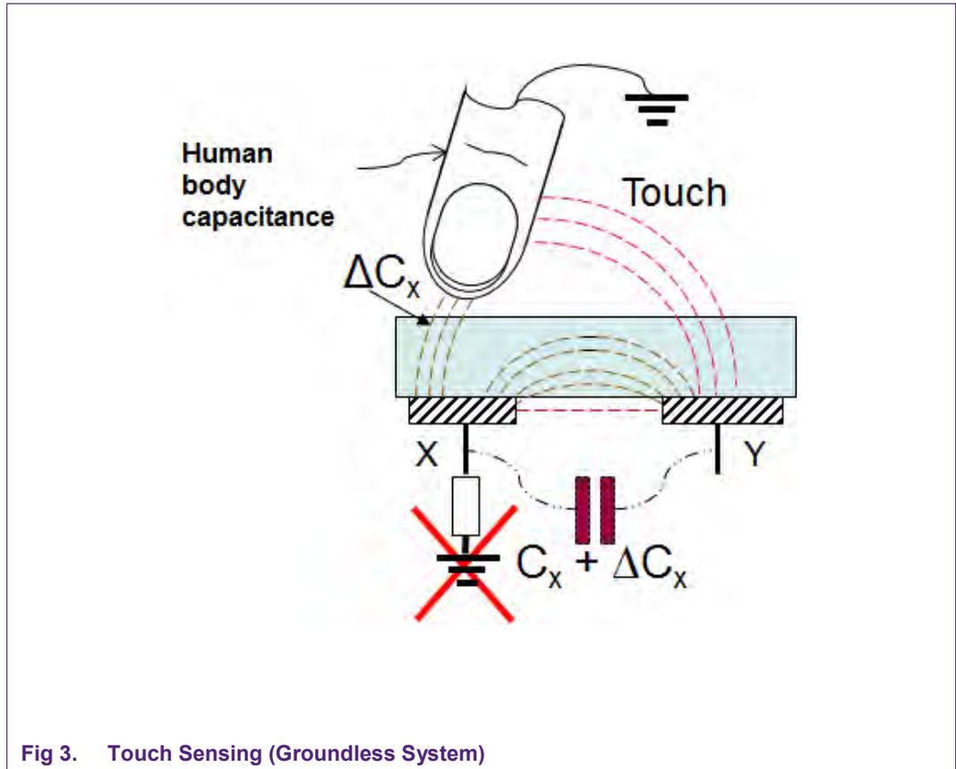
This very small relative change ( $-\Delta C_x$  or  $+\Delta C_x$ ) in the sensor capacitance is detected as a Touch. In addition, there's a lot of post processing involved to increase the robustness, to filter out the noise/jitter, to control the sensitivity, and to compensate for the environmental changes, such as, change in humidity, temperature, or operating voltage.
