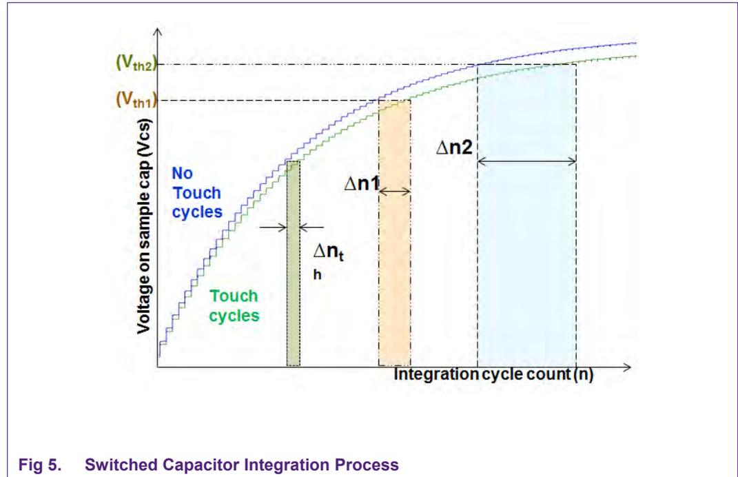
Fig 5. Switched Capacitor Integration Process
