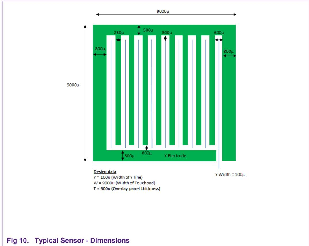
Fig 10. Typical Sensor - Dimensions
